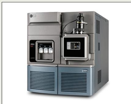
Each Waters Xevo MS features a universal ion source architecture: interchangeable ion sources that can be fitted to, or removed from, the face of the MS in minutes, without the need to shut down the system. This has changed the way analytical scientists working in high-throughput labs, and with little previous MS experience, can maximize the performance and productivity of their instrumentation.
