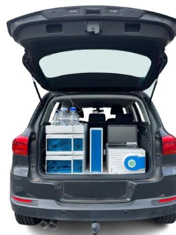
FIGURE 1 Full system shown for the work presented. Left: Automated Online SPE-LC Pump System, middle: Column Thermostat, Right: Microsaic 4500 MiD® Mass Spectrometer. The resulting small footprint allows for it to be fully deployable and at the point-of-need.
