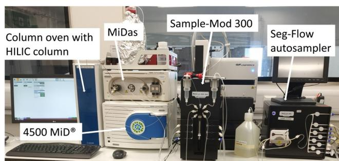
**FIGURE 1:** Experimental configuration of the Microsaic Metabolite Monitoring PAT system – The autosampler, consisting of a Seg-Flow autosampler coupled to a Sample-Mod 300 (right), sampled from the 10 L bioreactor at a pre-defined time interval and delivered these filtered cell culture samples to the 1 µL injection loop on the MiDas™ equipped with a ceramic pump head (left). Samples were separated using HILIC chromatography prior to analysis by the point-of-need 4500 MiD®
