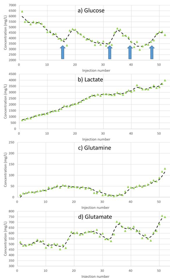
**FIGURE 3:** Metabolite concentration profiles during the 10 L cell culture when testing the Microsaic Metabolite Monitoring PAT system. Glucose feeding (large bolus) interventions are shown as arrows
