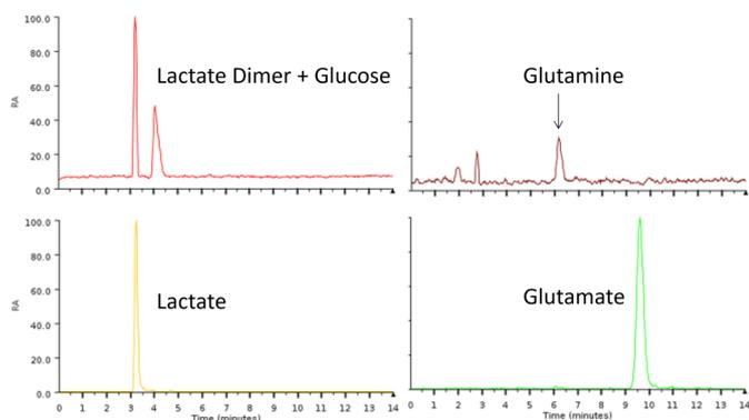
**FIGURE 2:** Typical chromatogram showing the simultaneous metabolite profiling of the filtered cell broth sample delivered from the bioreactor via the autosampler.
